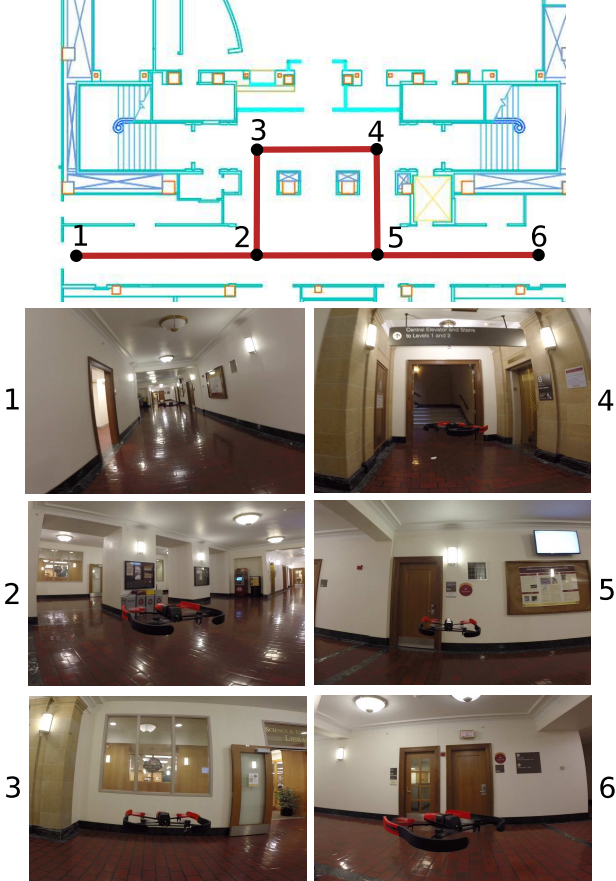
Figure 9. Experiments Set 1: (Top) Blueprint of the experimental area with the reference trajectory (1-...-6-1) overlaid. (Bottom) Snapshots of the Bebop along its path (locations 1-6).
