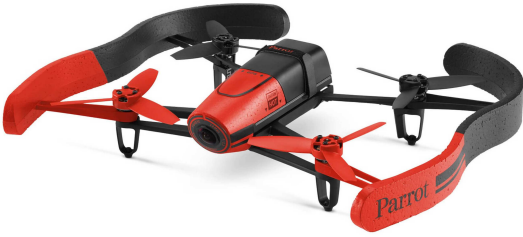
Figure 1. The Parrot Bebop quadrotor equipped with a 180 deg wide field of view (WFOV) camera, an optical-flow sensor, and an ARM-based processor.
