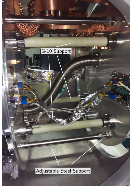
Figure 7. Image of G-10 and adjustable supports in the first 90 GHz receiver. The G-10 supports add significant stiffness – reducing the movement of the 4 K baseplate due to the weight of the shell and optics by a factor of five – but they add only 0.25 W of conductive power to the 4 K stage.
