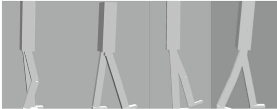
Fig. 1. Simplified gait cycle for right leg
