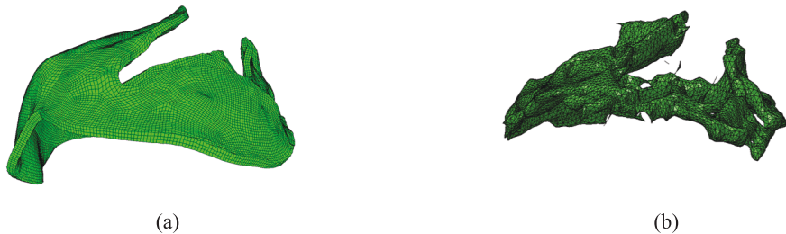
FIG. 8. Comparison of leaflet shapes at MV opening: (a) the complex model at time 0.615 s and (b) the segmented MV data from CT scan.
