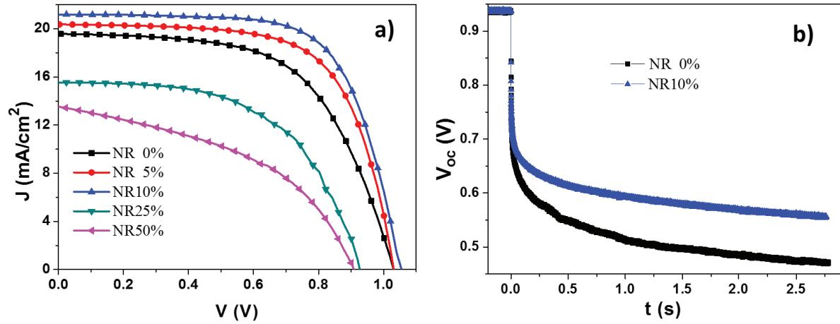
**Figure 6:** (a) J-V characteristic of the fabricated PSCs based on five different scaffold structures under one standard solar light illumination. (b)  $V_{oc}$  decay measurement for two representative cells. The monochromatic light illumination was turned off at  $t = 0$ .
