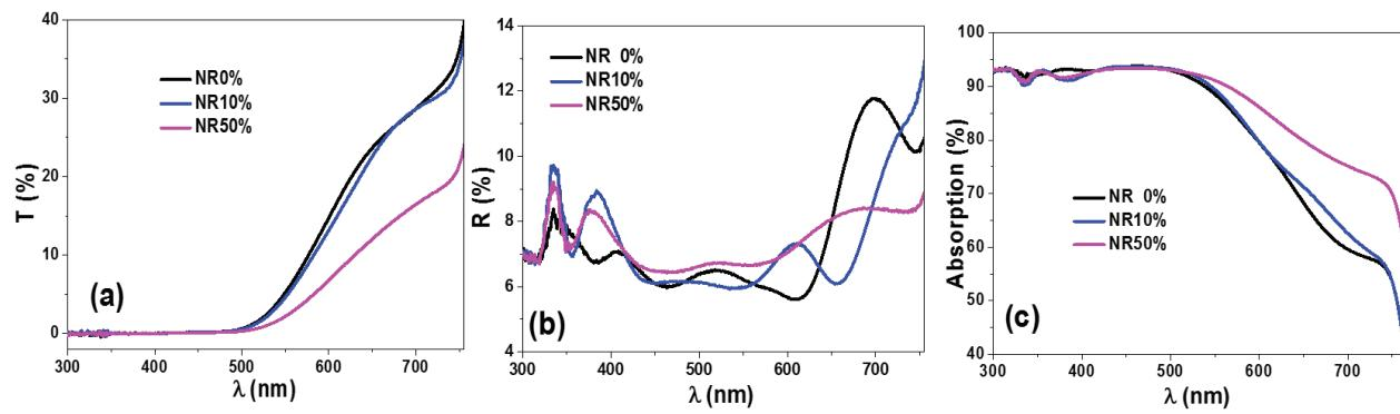
**Figure 4.** The transmission (a), reflectance (b), and absorption (c) of three representative samples NR0%, NR10%, and NR50% infiltrated with perovskite, were measured by an integrating sphere with light incidence from FTO glass side.
