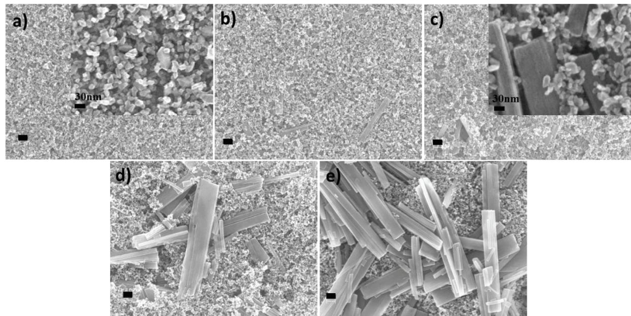
**Figure 3.** SEM images to compare surface morphology of the five porous TiO<sub>2</sub> scaffolds: a) pure NPs (0% NRs), b) 5% NRs, c) 10% NRs, d) 25% NRs, and e) 50% NRs. All images have a scale bar of 100 nm. The insets in a) and c) show the detailed surface morphology of 0% and 10% NR based scaffolds, respectively.
