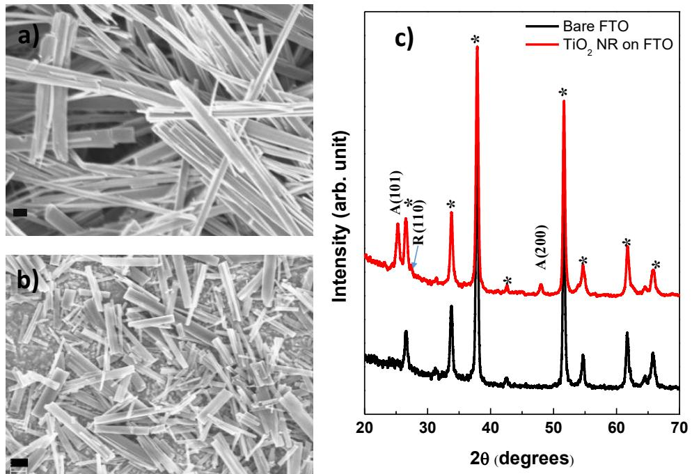
**Figure 2.** SEM images of long nanobelts/nanowires in (a) and short nanorods in (b). (Black scale bar: 300 nm). (c) XRD pattern of TiO<sub>2</sub> NRs dispersed on FTO glass substrate indicates the dominant anatase phase with tiny rutile inclusion. (\*: peaks from FTO substrate. A: anatase, R: rutile).
