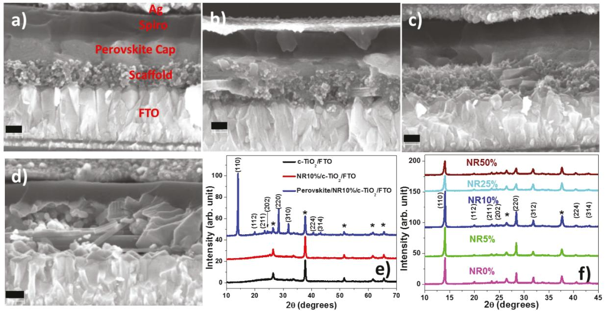
**Figure 5:** (a-d) Cross-section SEM of the fabricated PSCs based on scaffolds made of 0%, 5%, 10%, and 50% NR. (Black scale bar: 100 nm). (e) XRD pattern of the infiltrated perovskite material as well as those of the compact  $\text{TiO}_2$  layer and a scaffold layer made up of 10% NR. (f) Comparison of the XRD patterns and diffraction intensities of perovskite formed on all five different scaffolds. (\* represents FTO peaks).
