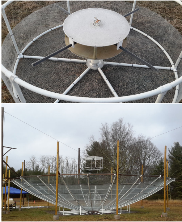
Fig. 1 Top: The HERA feed consists of a pair of crossed-dipoles over 1.72 m diameter backplane made of wire mesh. The backplane is surrounded by 0.36 m wide wire mesh around the edge resulting in encasing the crossed-dipoles in a cylindrical cage. Bottom: A prototype HERA element at the Green Bank NRAO site consisting of a crossed dipole feed and a paraboloidal reflector dish
