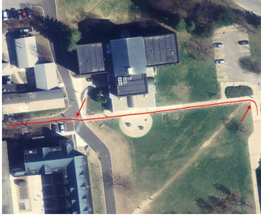
Figure 6: Position tracked by Tango overlaid on satellite imagery corresponding to its global position. Notice that the recorded position stays within the footpath. Arrows indicate both a subtle change in the linear-route (left) and a curve (right) that are not detectable with current wheel-encoder based GPR.
