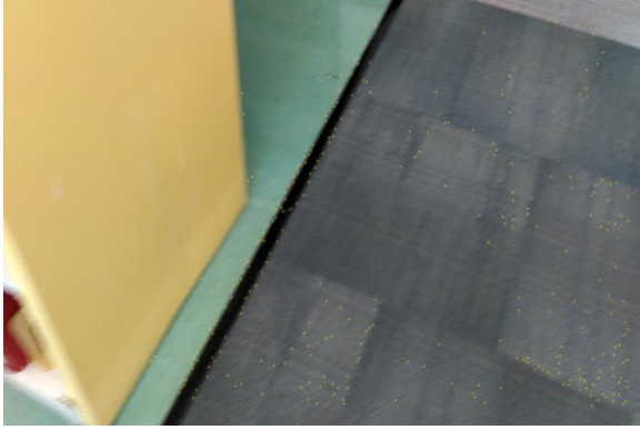
Figure 4: Tango feature points (yellow dots) detected using its fish-eye and RGB cameras.
