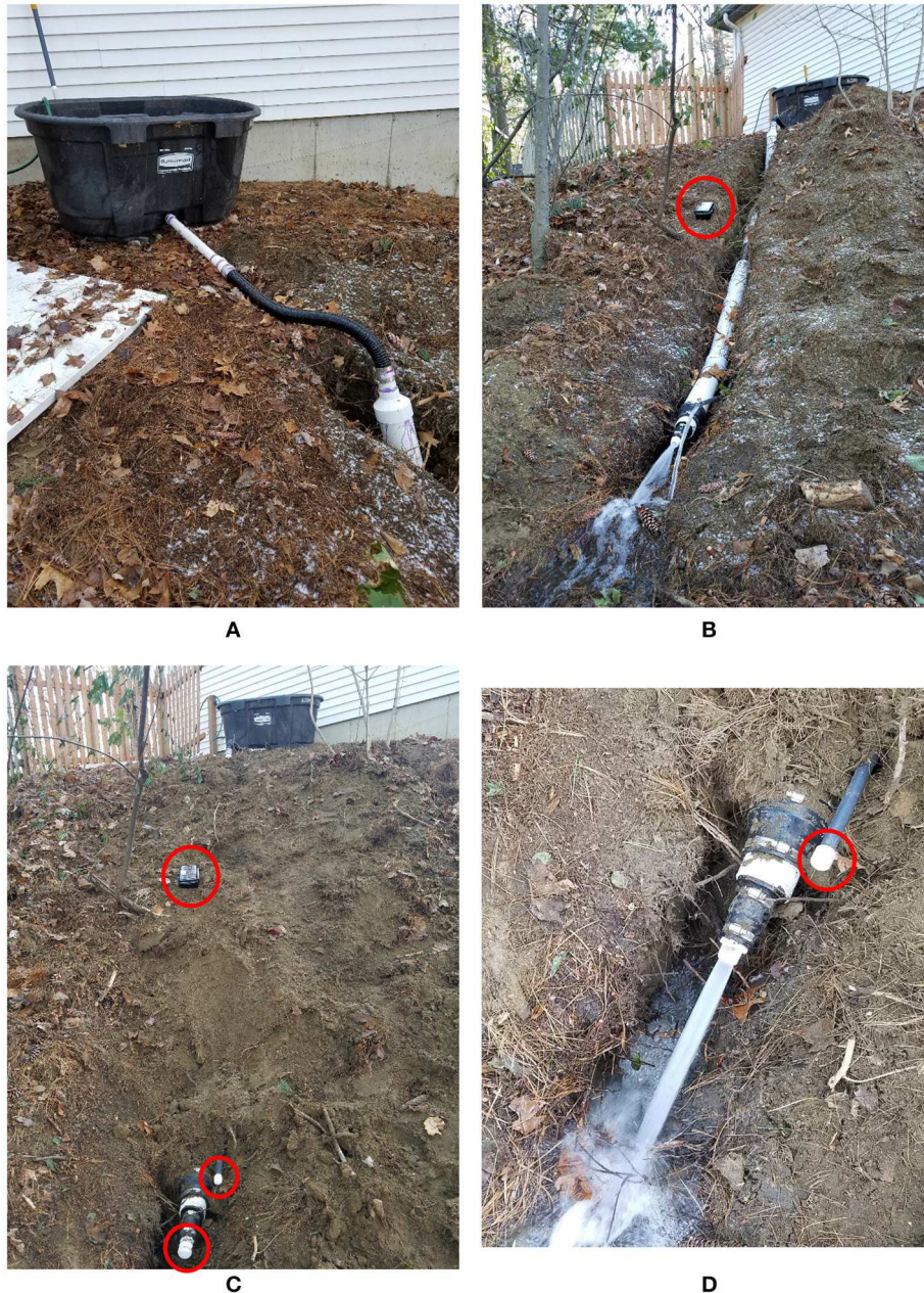
FIGURE 18 | (A) Rain barrel water source for buried pipe containing rotating magnet flow meter. (B) Pipe containing rotating magnet flow meter before burial. Arduino Mega unit with magnetometer and LoRa transmitter is indicated. (C) Pipe after burial. The Arduino Mega unit and the pipe's two drain outlets are circled in red. (D) Water drains through the larger of the two drain outlets. The smaller drain outlet is circled in red.
