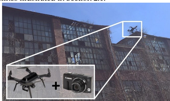
Figure 5. Image collection using an UAV (3DR Solo Quadcopter) with a consumer-grade camera (Canon PowerShot SX280).
