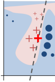
Figure 4: The intuition underlying constructing an approximate, locally linear model. “The black-box model’s coefficients (known to LIME) are represented by the size of the bold red cross is the instance being explained, gets predictions based on its proximity to the instance being explained (by size). The dashed line is the locally (but not globally) fitted model.”
