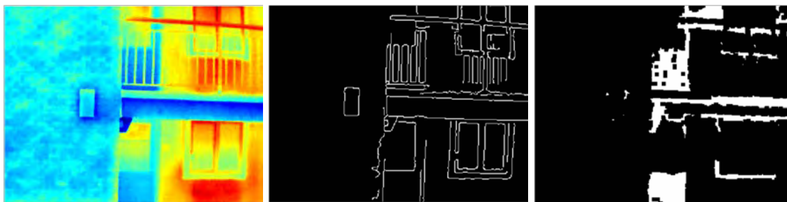
c) False positive detection of infiltration and missing envelope deterioration.
