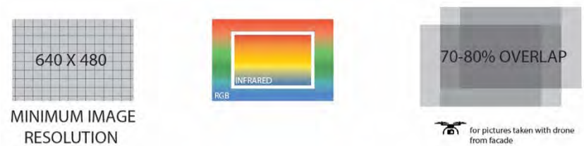
Figure 2 - In-flight imaging procedure for possible dual cameras, demonstrating target % overlap for auditing purposes.
