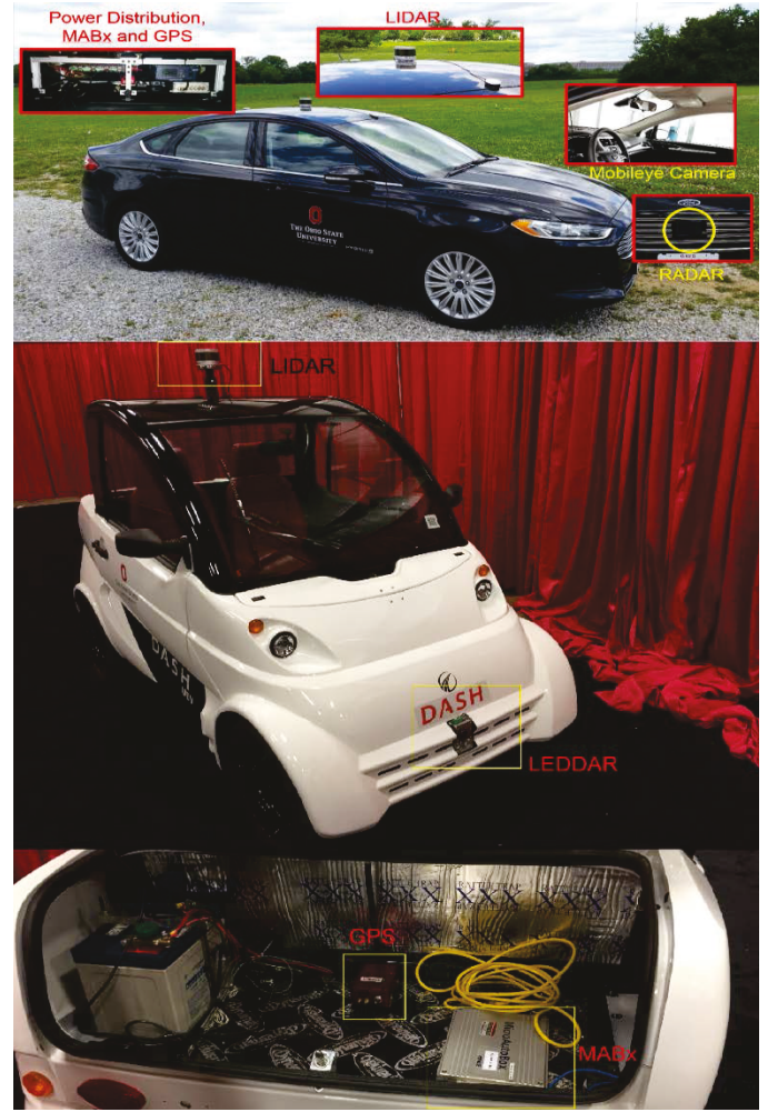
Fig. 2. Implementation of sensors and electronic control unit in both vehicles.
