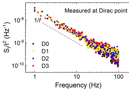
**Fig. 5:** Normalized current noise spectral density  $S_I/I^2$  at the Dirac point measured after each irradiation step. The  $S_I/I^2$  remains unchanged at various irradiation levels. Mobility fluctuation model can fully explains this trend.
