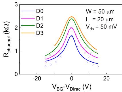
**Fig. 3:** Intrinsic channel resistance of the graphene/h-BN FET as a function of the back-gate voltage measured after each irradiation step. The solid lines represent the measured results and the open circles represent the fitted data.
