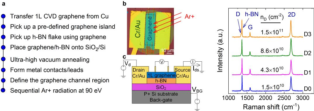
**Fig. 1:** (a) Key fabrication steps of the graphene/h-BN FETs. (b) Optical image of the final four-point structure. Multiple steps of low energy  $\text{Ar}^+$  irradiation were performed to introduce different densities of single vacancies in the graphene channel. (c) Schematic illustration of the measurement setup.
