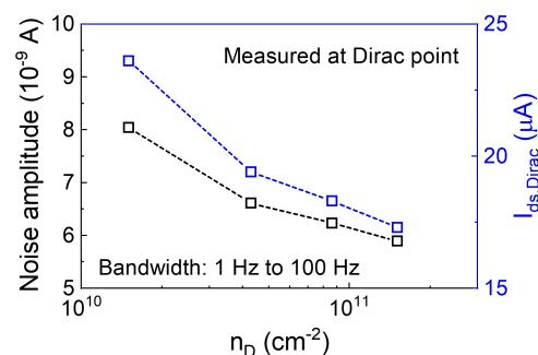
**Fig. 6:** Noise amplitude and drain current at the Dirac point vs. concentration of vanacy defects  $n_D$ . Noise amplitude decreases in proportion to  $I_{dS, \text{Dirac}}$ .
