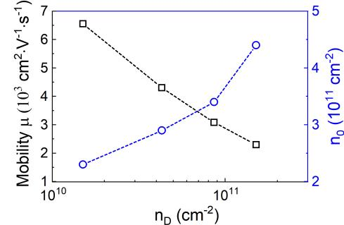
**Fig. 4:** Carrier mobility  $\mu$  and the residual carrier concentration  $n_0$  vs. defect density  $n_D$ . The lines are guide to the eye.
