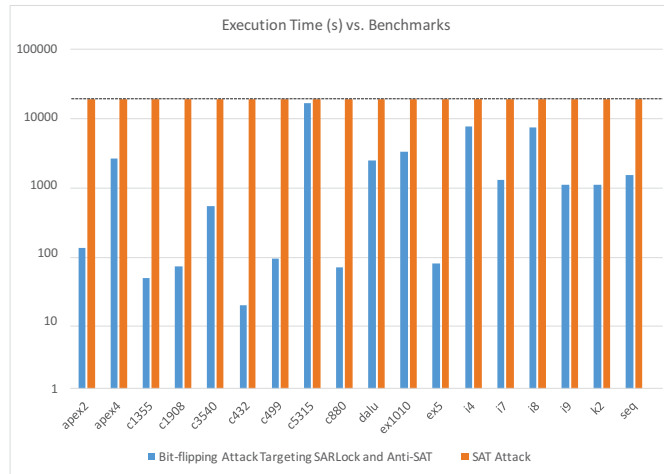
Fig. 4. Execution time of performing the SAT attack and bit-flipping attack targeting SARLock and Anti-SAT on benchmarks encrypted with RND + Anti-SAT (5% overhead).
