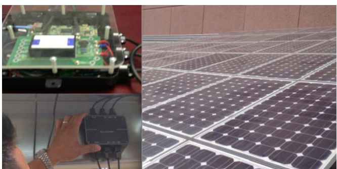
Figure 2. The solar energy monitoring facility at ASU showing the sensor fusion center, the smart monitoring device, and the solar panels. One SMD is dedicated for each solar panel rendering it as an IoT programmable node.
