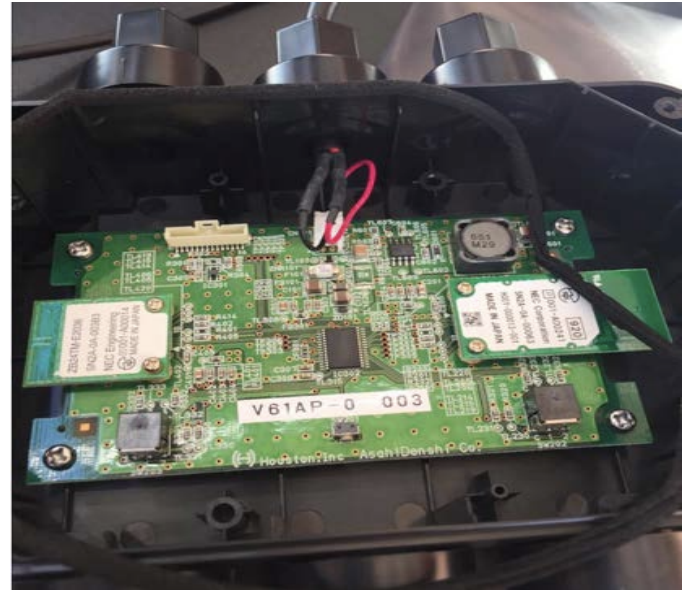
Fig. 1. Smart monitoring devices (SMDs) developed in Japan and used for Solar monitoring and control research. The SMD has a microcontroller, a network radio, relays for reconnecting or bypassing panels, and sensors. With the SMDs, solar panels are seen and managed as IoT nodes.
