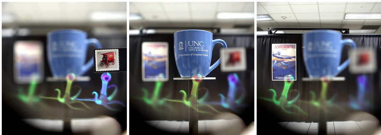
Figure 1: Images looking through our varifocal display prototype showing 3 real world objects (top) and 3 virtual aliens (bottom) at 3 different depths: 20 cm (stamp and blue alien), 50 cm (mug and yellow alien), 800 cm (poster and green alien). Virtual objects not at current focal depth are computationally blurred.
