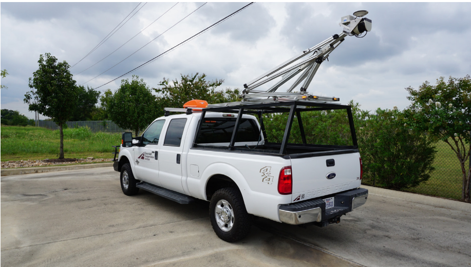
Fig. 2. MLS used in data collection, consisting of SICK LMS-5XX laser scanner, GPS Unit, IMU, forward looking video camera, and data storage and processing systems.
