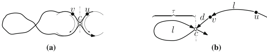
Fig. 9 a The length of the tie to the left of the dash-dotted vertical line is equal to the length of the section of ring from u to v . b The robots u and v prevent each other from starving because the distance between them is equal to the length of a tie in the same ring
