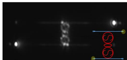
Figure 3 Intensity profile of resonators comprised of two microrings coupled through an intermediate link cavity.
