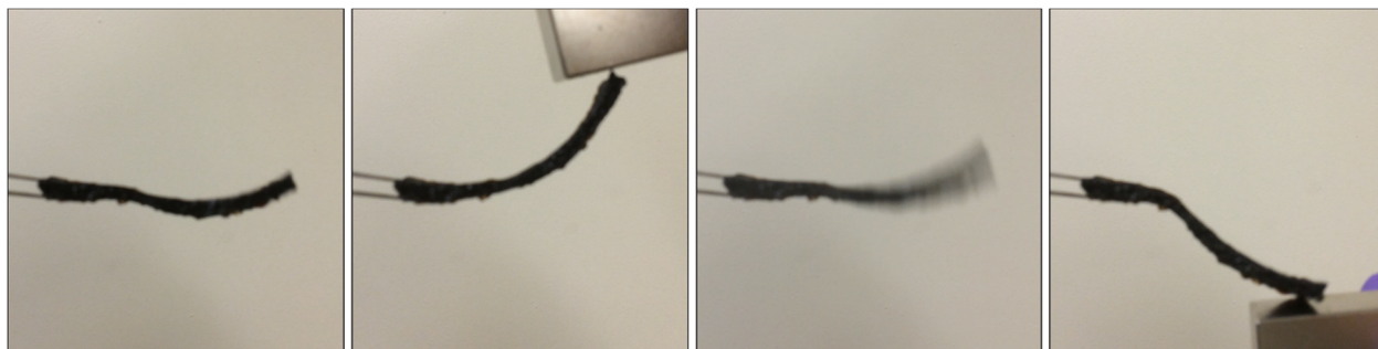
Figure 7. Bending of a hydrogel bar (length ~ 6.5 cm, 71.5 wt% water) of sample (PES/Co) 19 -EO 800 -(PES/Co) 19 by a neodymium magnet.
