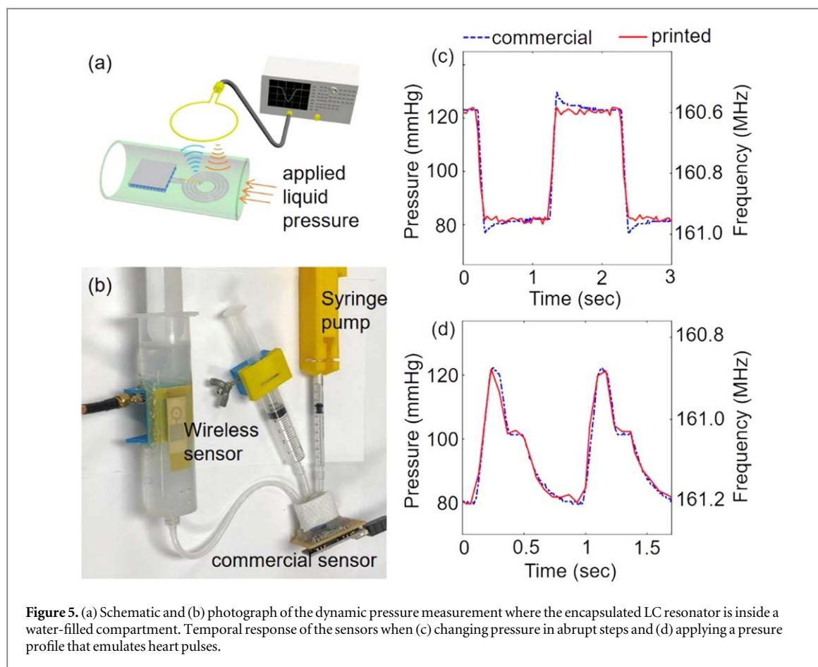
**Figure 5.** (a) Schematic and (b) photograph of the dynamic pressure measurement where the encapsulated LC resonator is inside a water-filled compartment. Temporal response of the sensors when (c) changing pressure in abrupt steps and (d) applying a pressure profile that emulates heart pulses.
