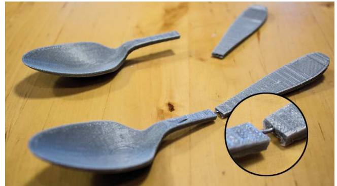
Figure 8. Embedding wire straightened from a paper clip into a spoon avoids snapping, which could be dangerous to the user during breakage. Please also see our accompanying video figure.
