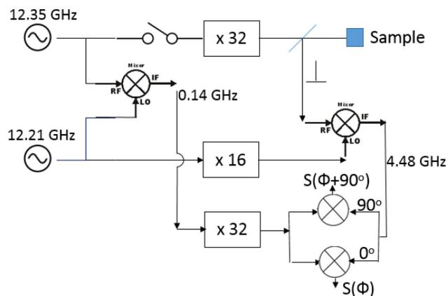
Fig. 1. Schematic setup for pulsed EPR at 395 GHz, with quadrature detection.  $S(\Phi)$  and  $S(\Phi+90^\circ)$  are the final signals that allow for simultaneous detection of absorptive and dispersive components in a digital oscilloscope.
