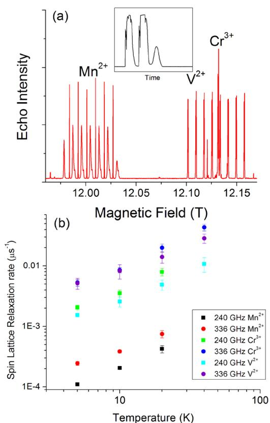
Fig. 3. (a) 336 GHz echo detected EPR spectrum of impurities in a MgO substrate at 20 K. The inset shows a 2-pulse Hahn echo sequence followed by the response from the spin system (echo). (b) Spin-lattice relaxation rates for impurities in MgO at 240 and 336 GHz.
