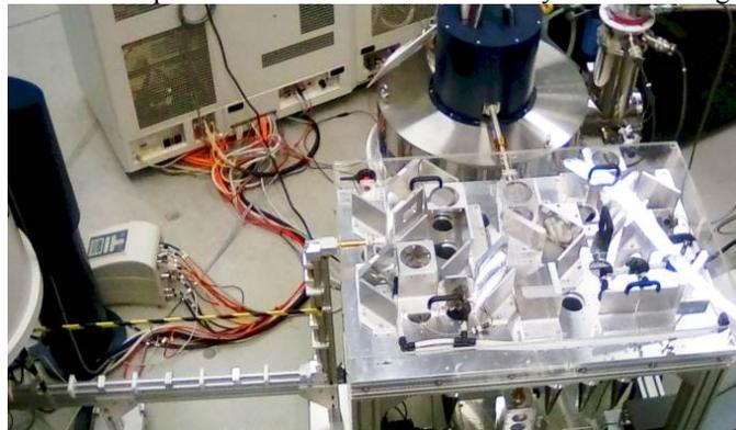
Fig. 2. Quasi-optical table for DNP, with the gyrotron source in the upper right and the NMR magnet on the left.
