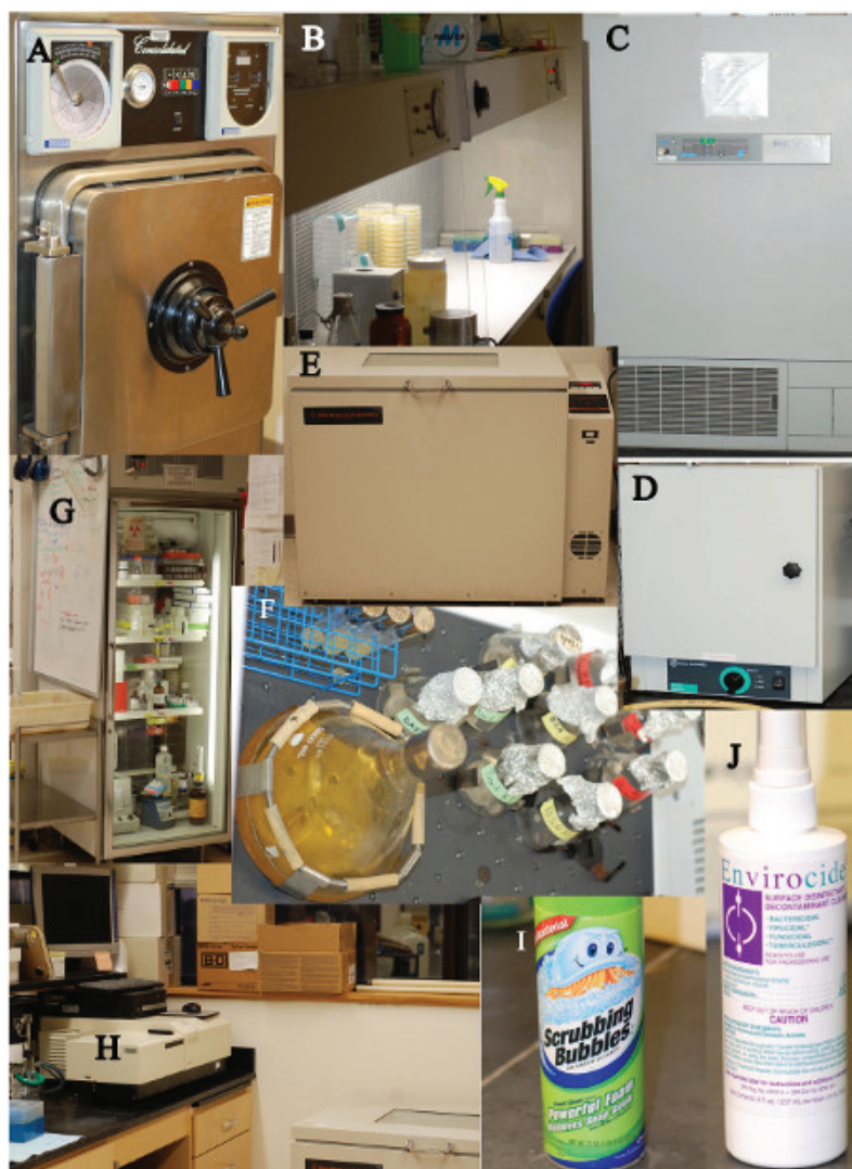
Figure 2. Some of the equipment and material necessary for performing phage display. Sterile technique requires access to both: A) an autoclave and; B) a laminar flow hood. Phage libraries and BLT5403 bacterial stock require -80^{\circ}\text{C} temperatures for prolonged storage C) Growing phage and bacteria requires, D-F) 37^{\circ}\text{C} incubators, one of which, E-F) is capable of growing liquid cultures (orbital). Optimizing the experiment through color coding, F) minimizes mistakes. BLT5403 cells for titering can be stored for up to one week, G) at 4^{\circ}\text{C} . Optimizing the placement of the, H) spectrophotometer for following cell densities next to the orbiting shaker can save time. Frequently treating surfaces and pipets with, I) powerful detergent and J) Enviroid, can help to minimize the risk of viral contamination.
