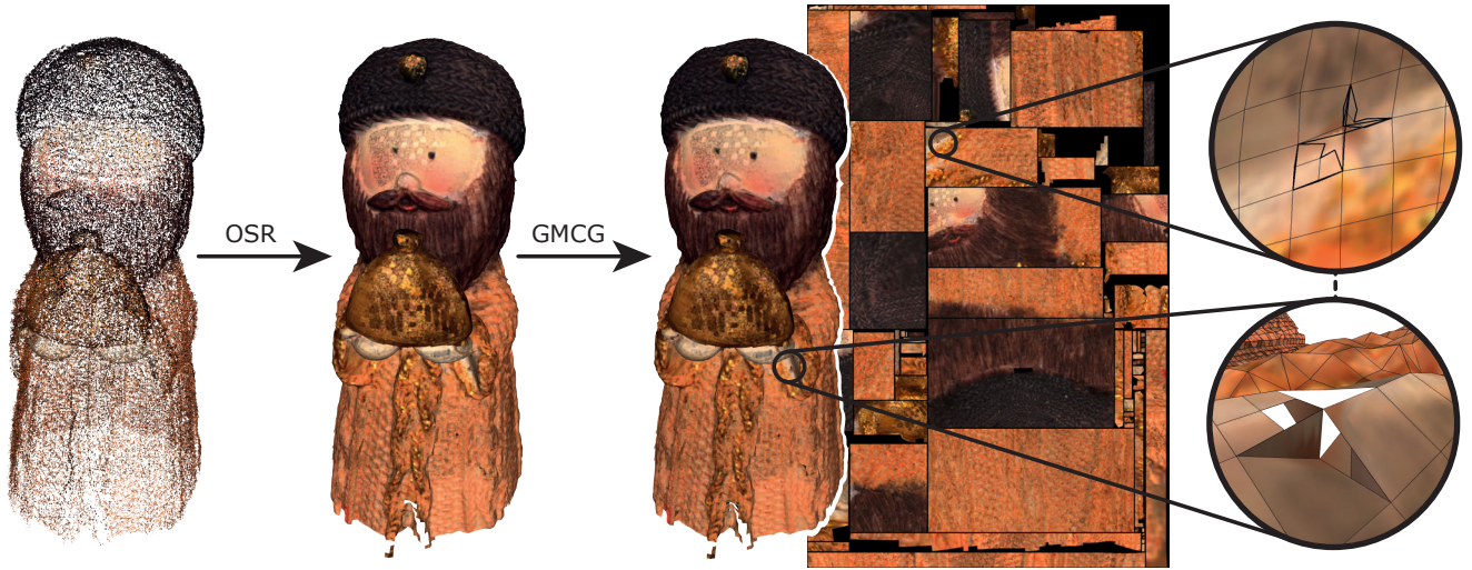
Fig. 18. Parametrization by Generalized Motorcycle Graphs close the gap between meshing approaches like Online Surface Reconstruction (OSR) and many applications that use standard textured meshes as input. OSR takes several point clouds as input (left) and produces a semi-regular mesh in a specialized format (middle). Natural Motorcycle Graphs can generate a standard textured mesh (right) from this format. To support this application, it is imperative that Natural Motorcycle Graphs handle imperfections in the input data (highlighted areas) and produce a practically usable texture map.
