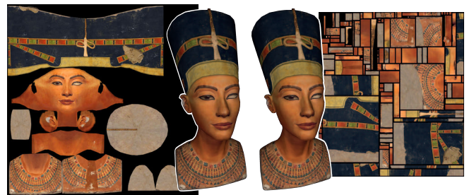
Fig. 21. Generalized Motorcycle Graphs can be used to resample and repack textures of a hand-made model (left) to a denser texture (right). In this example, texture occupancy increased from 64.3% to 97.9%.
