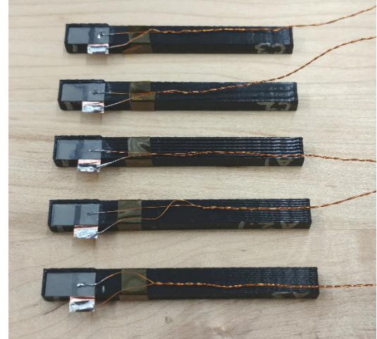
Figure 3. Test specimens instrumented with piezoelectric transducers.
