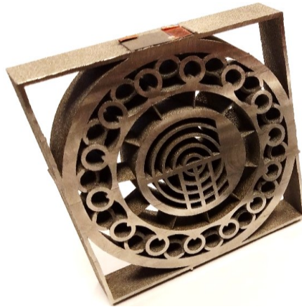
Figure 3. Baseline specimen after bottom machining removal and post-second EMI testing. A PZT is seen attached on the top.
