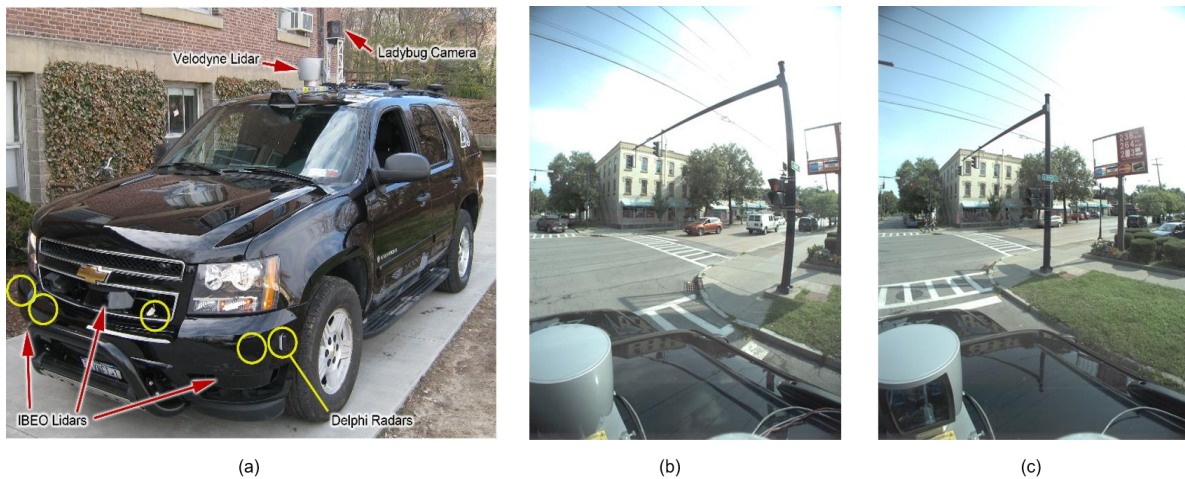
Fig. 7. (a) Test vehicle with notable sensors indicated; note only the Ladybug camera was used in this study, the lidar and radar units were not used. (b) Test image of a landmark from the Ladybug camera during the experiments. (c) Database image of the landmark corresponding to the image in (b). These images produced a match and resulted in a landmark measurement update despite being taken on different days under different conditions. Note the resolution of the original images is 1232 x 1616
