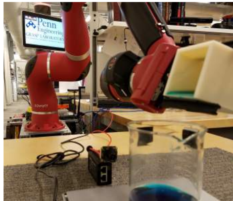
Fig. 1: Experimental setup using the Rethink Robotics Sawyer manipulator to pour precise amounts of water into a beaker using vision for feedback control.
