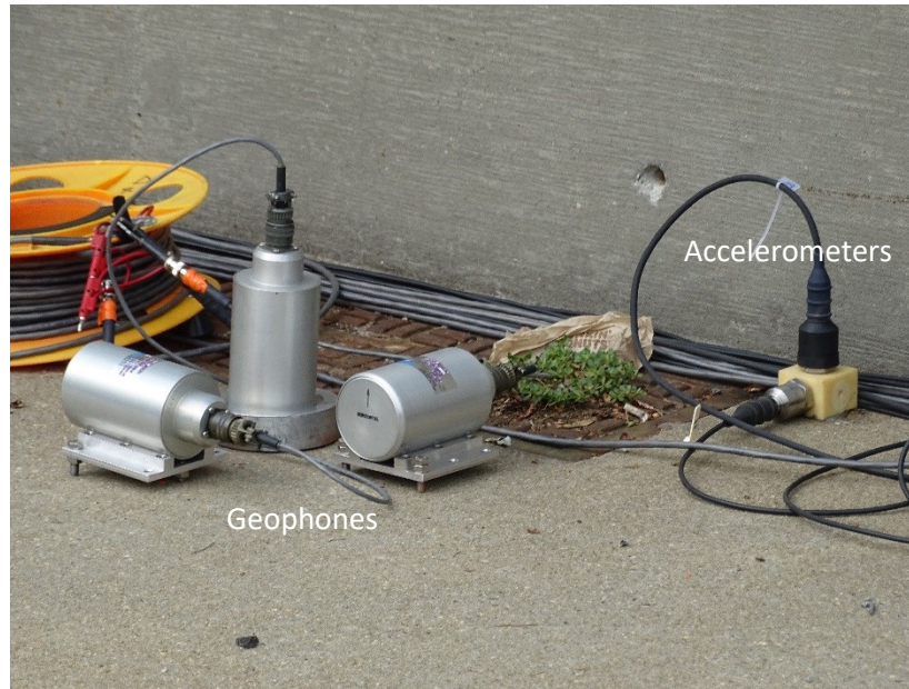
Figure 5: Geophone and accelerometer arrays used to capture the dynamic response.
