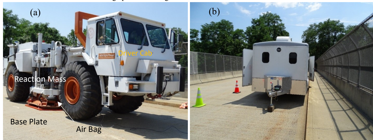
Figure 3: (a) T-Rex on bridge. (b) Control room to monitor response in real-time.
