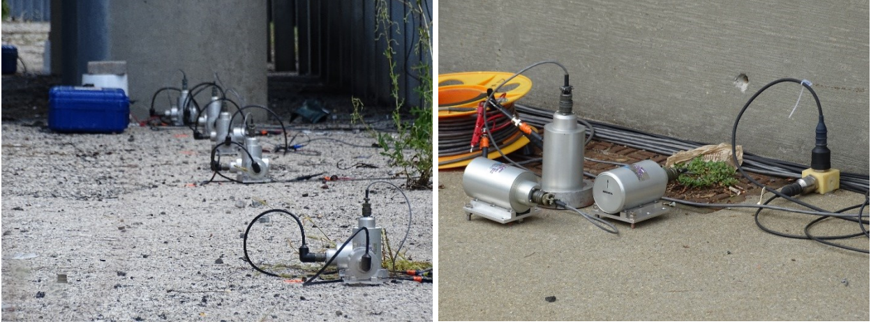
Figure 3. On the ground geophone arrays (left) and geophone and accelerometer array on the deck (right).
