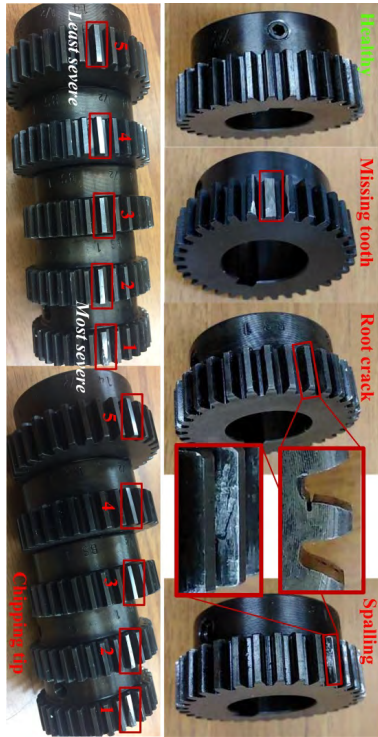
FIGURE 8. Nine pinions with different health conditions (five levels of severity for chipping tip).
