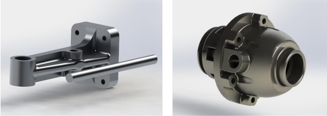
Figure 5. Part designs considered in the case studies. Aluminum bearing bracket (left), and steel gearbox housing (right).
