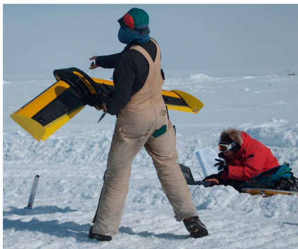
Fig. 1. Launch of our QUEST 300 UAV. The catapult launch line extends 20 m to the left of the photo and is anchored in the snow. Ground control is via laptop computer with telemetry. Photo: Stephanie Wissel.
