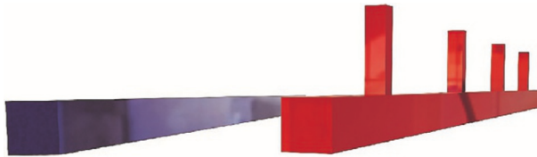
Fig. 26 Numerical models of the two experimental structures: the unpillared beam ( left ) and the pillared beam ( right ).
