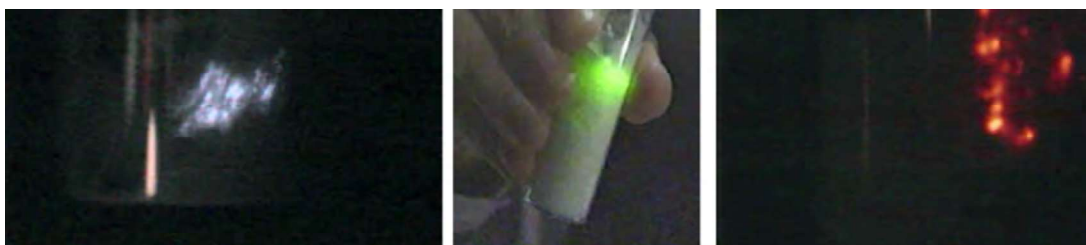
Figure 1. Examples of light emissions from highly efficient triboluminescent materials (Sage et al., 2001).
