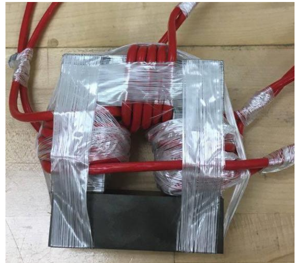
Fig. 5. Final assembled multi winding HF transformer
