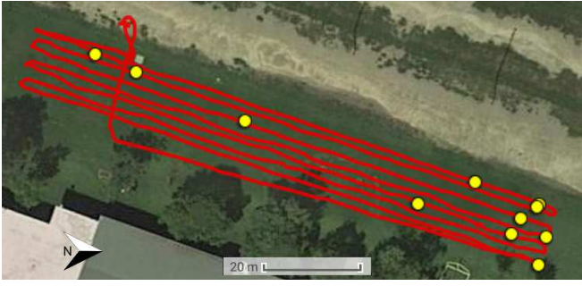
Fig. 11. The UAV's path for flight 3 is in red. Strikes collected along this path are represented by yellow dots.
