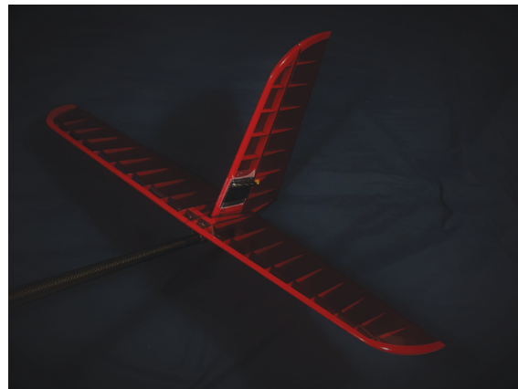
Figure 5. The tail of the UIUC Solar Flyer airframe, with a full-moving horizontal stabilizer.
