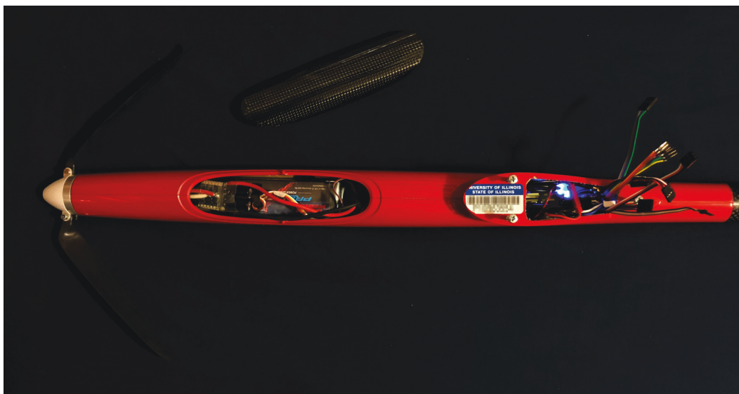
Figure 10. A photo of the top of the fuselage pod showing propulsion system elements in the front of the pod and the instrumentation in the rear of the pod; note that the wires connect to the sensors and flight control actuation system located in the wing.
