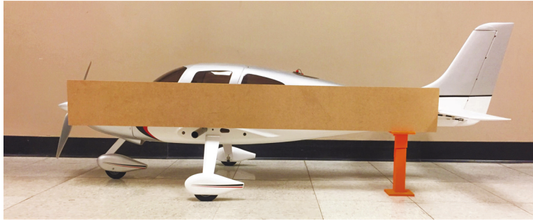
Figure 18. Area comparison of the Cirrus SR22T Baseline Testbed fuselage and the MDF flat plate.
