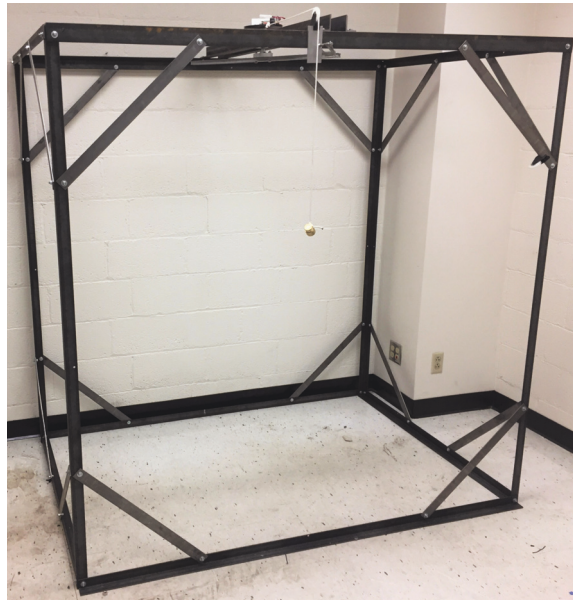
Figure 2. Moment of inertia measurement rig
