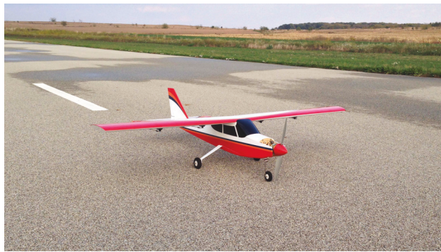
Figure 8: Flight-ready Avistar UAV used for the evaluation of the power model.
