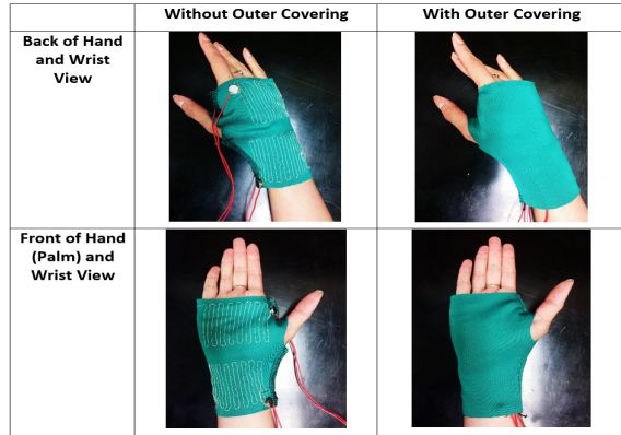
Figure 2: Garment Design: (Left) Inner lining of stitched resistive heating elements with (Right) Mylar insulation and additional polyester-spandex knit outer layer.
