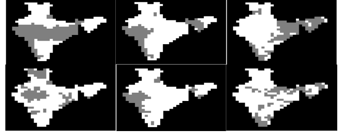
Fig. 3. Column 1: 1 August 2006, “active” by both MRF and [8], Column 2: 6 July 2006, “active” by [8] but normal by MRF, Column 3: 18 July 2007, “break” by [8] but normal by MRF. Top row shows locations assigned Z = 1 by MRF in grey, bottom row shows locations receiving more rainfall than their daily mean.
