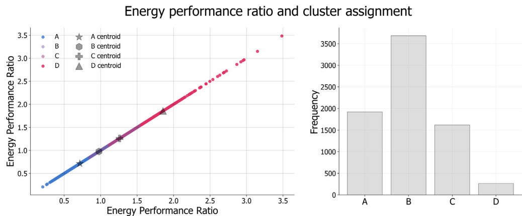
Fig. 4. Energy performance ratios, color-coded based on cluster assignment, and cluster centroids (left). Distribution of buildings assigned in each cluster (right).
