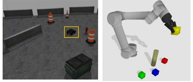
Figure 6: Simulation experiments. Left: Husky navigation task. The robot is highlighted. Right: UR5 block-stacking task with obstacle avoidance.
