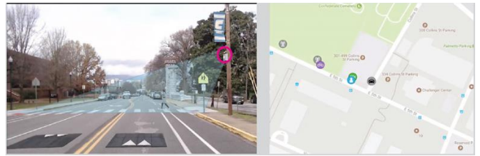
Figure 9. An infrastructure camera captures video from its field of view (left) and the information is displayed in real-time on the mapping application (right).
