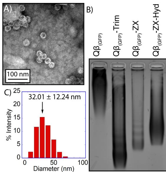
**Figure 3.** (A) TEM micrograph of the  $Q\beta_{(GFP)}\text{-ZX}$  conjugate. (B) Native agarose gel electrophoresis showing  $Q\beta$ ,  $Q\beta$  conjugates, and the hydrolyzed product  $Q\beta\text{-ZX-Hyd}$ . (C) DLS measurement of the  $Q\beta_{(GFP)}\text{-ZX}$  conjugate showing a uniform size distribution. The measurements were taken in KP buffer (0.1 M, pH 7.4, 25 °C) at concentrations of ~1 mg/mL.
