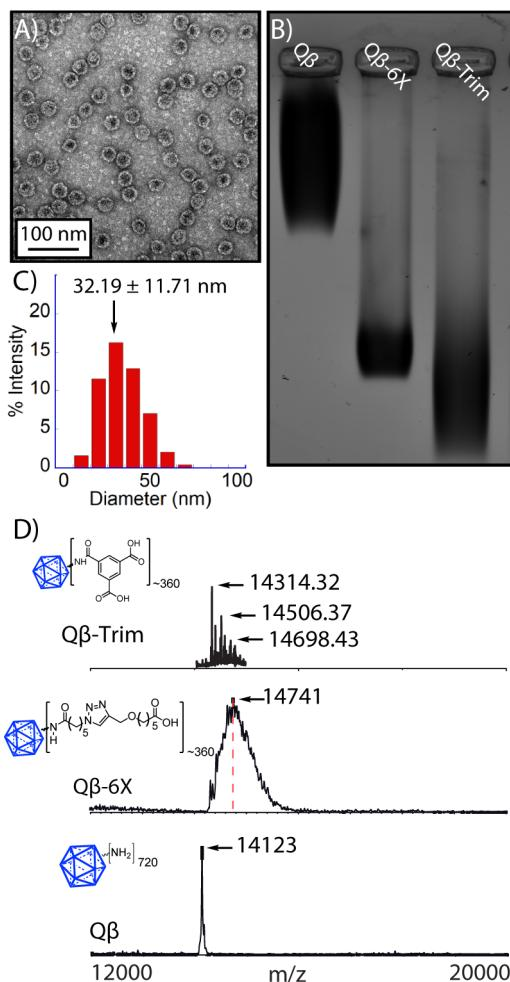
**Figure 1.** (A) TEM image of Q $\beta$ -6X. (B) Native agarose gel electrophoresis of Q $\beta$ , Q $\beta$ -6X, and Q $\beta$ -Trim. The greater mobility toward the positive electrode (bottom) suggests an increase in negative charge. (C) Dynamic light scattering data of Q $\beta$ -6X. (D) MALDI-TOF mass spectra of Q $\beta$  and Q $\beta$ -6X showing observed masses. ESI-TOF mass spectrum of Q $\beta$ -Trim showing one, two, and three functionalized residues per coat protein.
