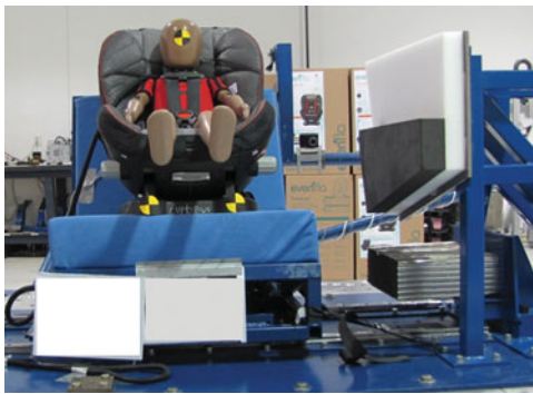
Figure 1. Sled set up using Takata side impact bench.
