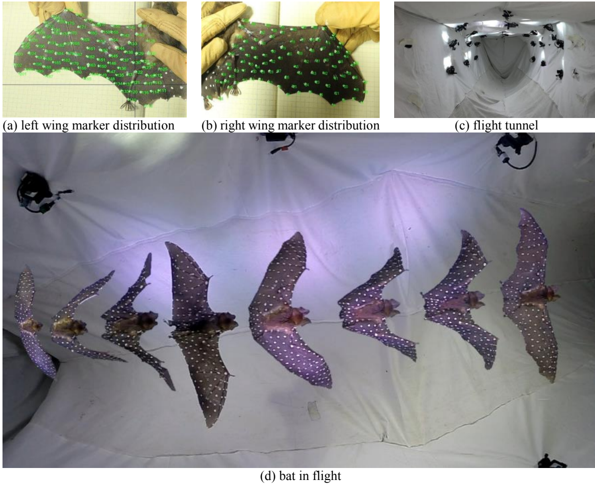
Figure 1. Motion capture experimental setup.
