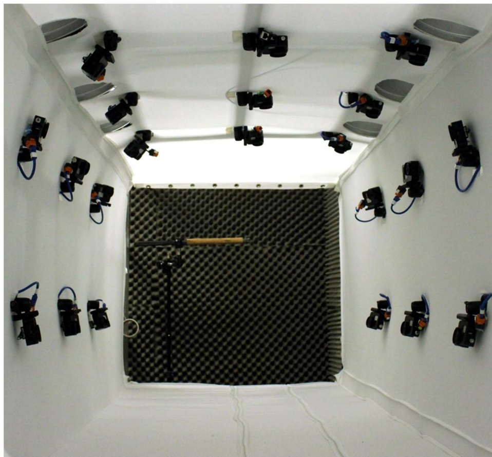
Fig 1. Motion capture system, consisting of 21 GoPro cameras inside a 1.2 x 1.2 meter cross section flight tunnel. The bat was trained to fly through the tunnel and land on the cork perch shown.
